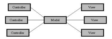
Fig. 3. The basic Model View Controller architecture
