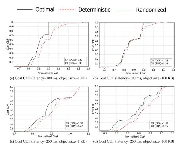
Figure 5.6: Cost performance of algorithms under tight and loose latency for objects with a replica. All costs are normalized to the local residential algorithm. The values in boxes show the CR of DOA and ROA in the worst case.
