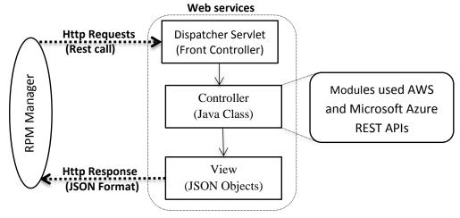
Figure 6.9: Web services components used in the prototype
