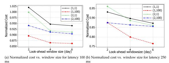
Figure 5.10: Normalized cost of the Randomized algorithm when the window size is varied. All costs are normalized to the local residential algorithm. Legend indicates replicas number and objects size in KB.
