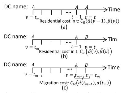
Figure 5.4: The description of Deterministic online algorithm. The residential cost of the object as if the requests on the object in slot v=t are served by (a) the determined DCs in time slot v-1 and (b) the determined DCs in time slot v. (c) The migration cost of the object between the determined DC in time slot  $v=t_{m-1}$  and  $t_m$ .
