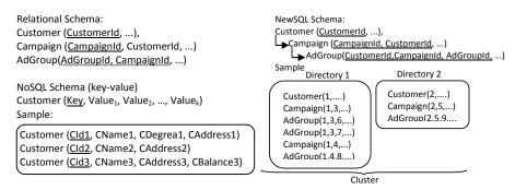
Figure 2.2: Relational schema and NoSQL schema with a sample
