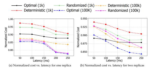
Figure 5.8: Normalized cost of algorithms when the latency is varied. Legend indicates object size in KB for different algorithms. All costs are normalized to the local residential algorithm.
