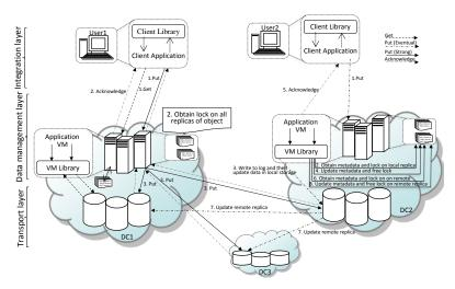
Figure 2.4: Inter-cloud storage architecture
