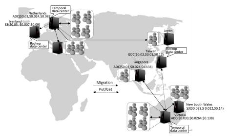
Figure 4.1: A scenario of the dual cloud-based storage architecture in the European and Asia-Pacific regions. Parenthesis close to each DC's name shows the storage price (per GB per month) for standard storage, backup storage, and network price (per GB), respectively.
