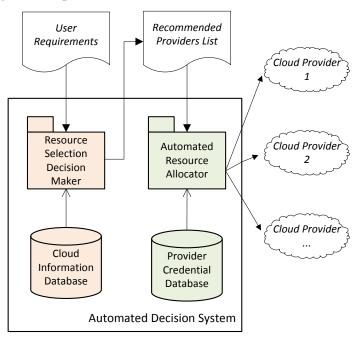
Figure 1 System Architecture of Automated Decision System
