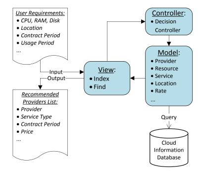
Figure 2 Resource Selection Decision Maker architecture of Model-View-Controller
