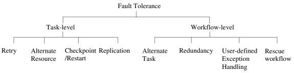
Figure 17. Fault Tolerance Taxonomy.
