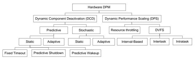
Figure 5. DPM techniques applied at the hardware and firmware levels.
