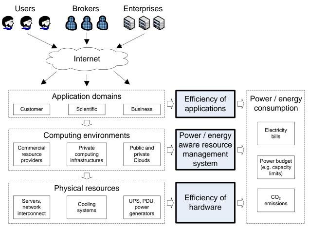
Figure 1. Energy consumption at different levels in computing systems.
