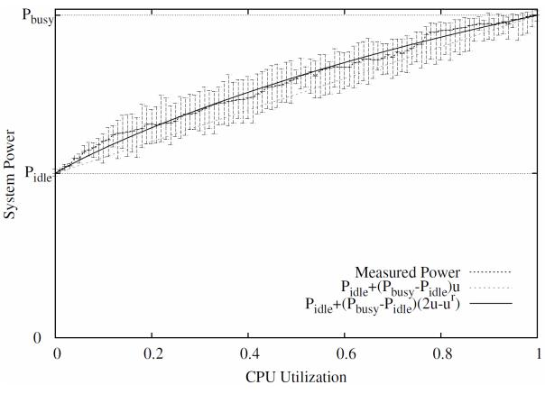
Figure 3. Power consumption to CPU utilization relationship [10].
