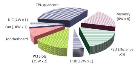
Figure 2. Power consumption by server's components [5].
