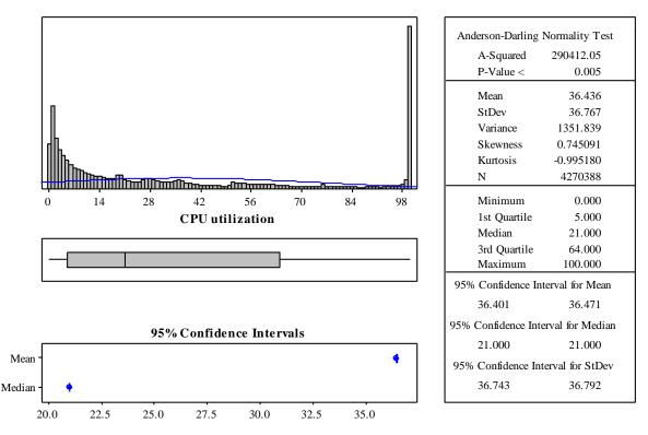
Figure 4. The CPU utilization of more than 1000 PlanetLab nodes over a period of 10 days.
