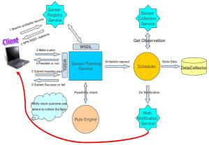
Fig. 7: Sensor Planning Service Architecture.
