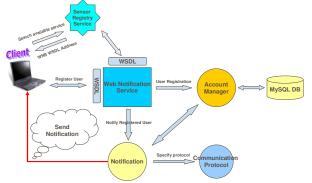
Fig. 8: Web Notification Service Architecture.
