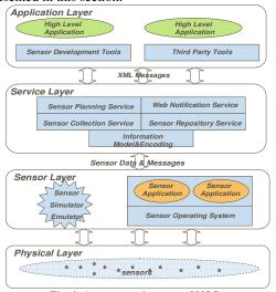
Fig. 4: A prototype instance of NOSA
