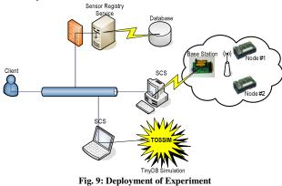
Fig. 9 illustrates the SCS as deployed on Apache Tomcat 5.0 server running on two different machines, one of which is hosting the TinyDB application under TOSSIM and the other the Temperature Monitoring application under Crossbow's motes. A Sensor Registry Service is also configured on a
