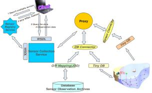
Fig. 6: Sensor Collection Service Architecture.
