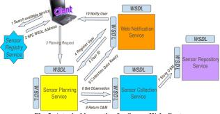
Fig. 5: A typical invocation for Sensor Web client.
