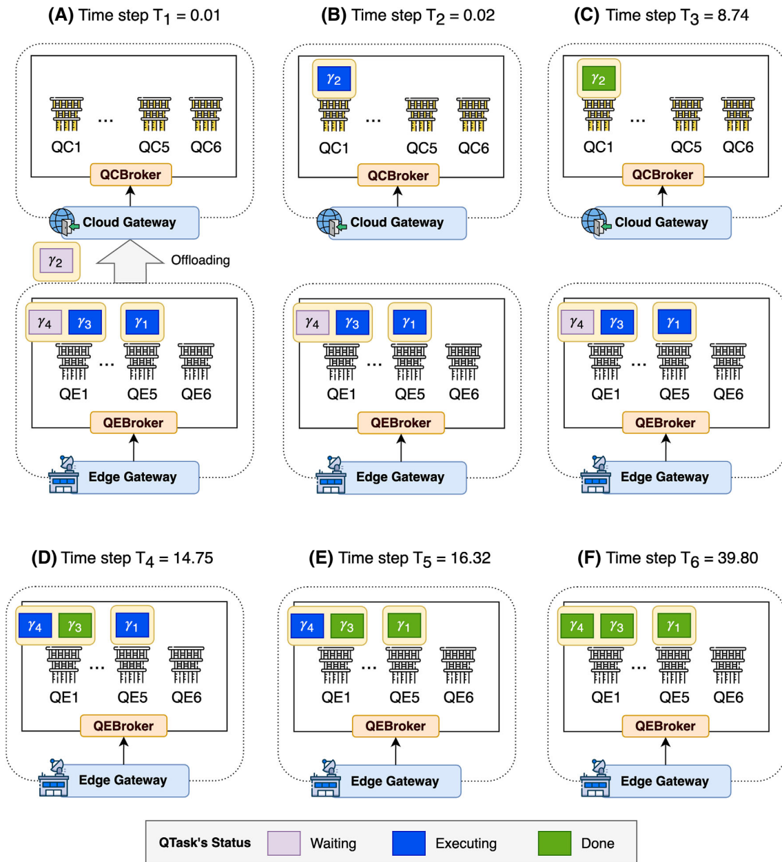
FIGURE 10 Dynamics of each time step involved in the verification process of iQuantum. The cloud layer in time steps T_4 , T_5 , and T_6 are truncated for simplicity as there are no new events after T_3 .
