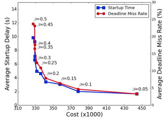
Fig. 9: Illustration of the Pareto front for determining the upper bound threshold ( $\beta$ ) in the dynamic provisioning policy. When  $\beta = 0.05$ , it produces the lowest startup delay and deadline miss rate at the highest cost. In contrast, when  $\beta = 0.5$ , it produces the highest startup delay and deadline miss rate at the lowest cost. There are values of  $\beta$  (*e.g.*, between 0.15 to 0.3) that provide low QoS violations with less incurred costs.
