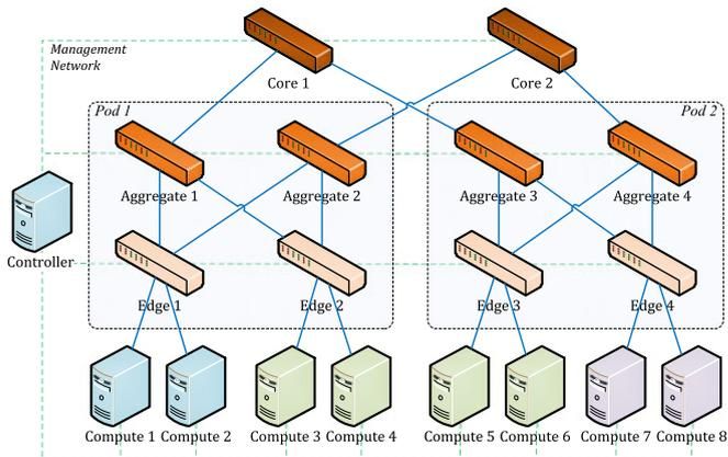
Fig. 5. Testbed configuration.
