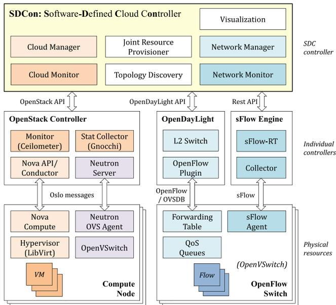
Fig. 2. System architecture of SDCon and underlying software components.
