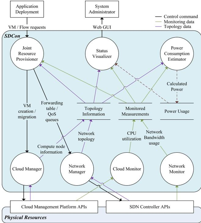
Fig. 3. Data flow diagram of SDCon components.
