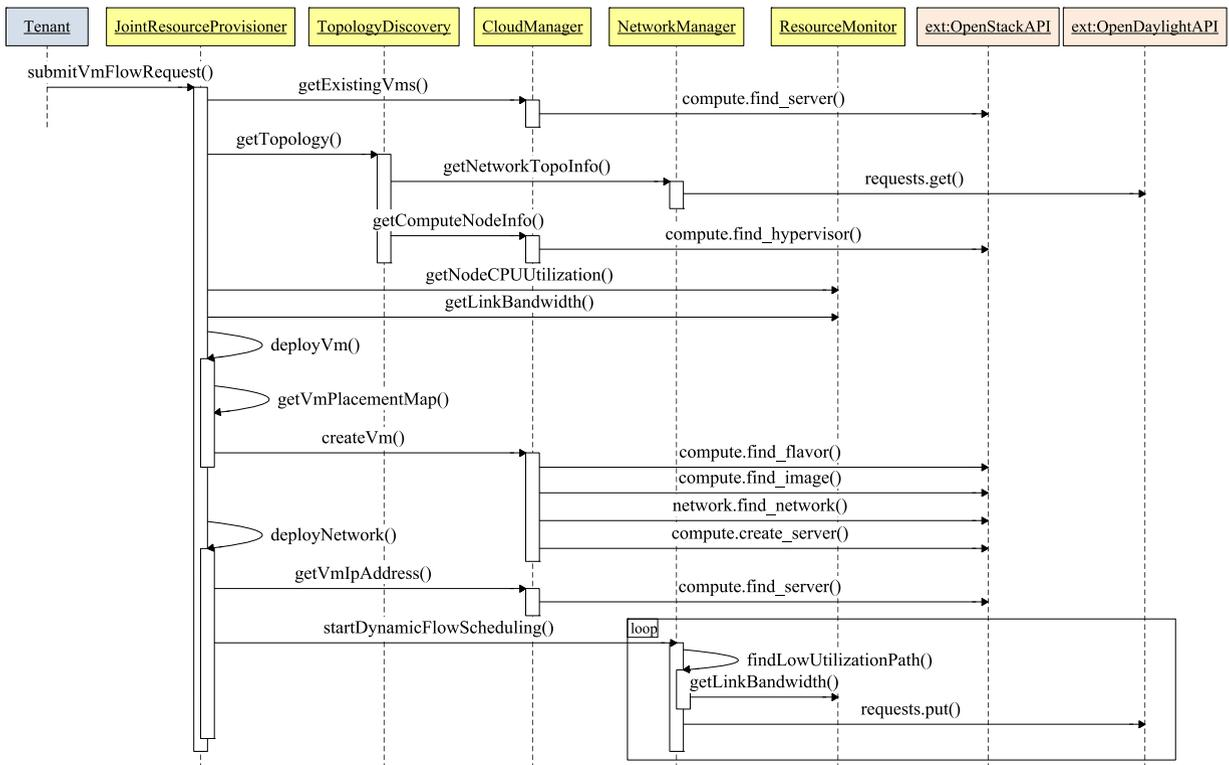
Fig. 4. Sequence diagram to deploy VMs and flows with SDCon.
