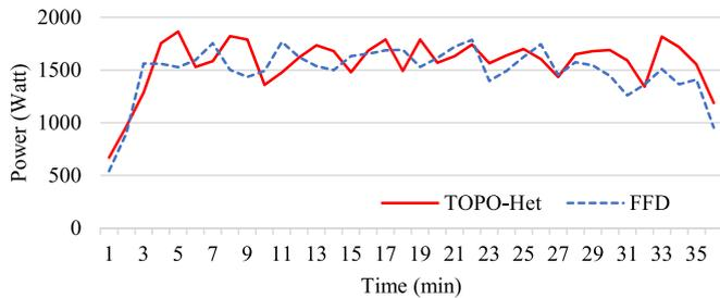
Fig. 11. Overall power usage of the testbed estimated from CPU and network utilization.
