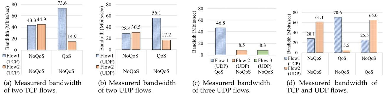
Fig. 6. Bandwidth measurement of multiple flows sharing the same network resource.
