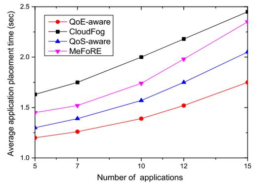
**Fig. 13.** Application placement time vs. number of applications.
