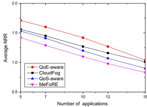
**Fig. 10.** Network relaxation ratio vs. number of applications.
