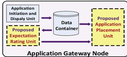
Fig. 3. Architecture of a Fog gateway node.
