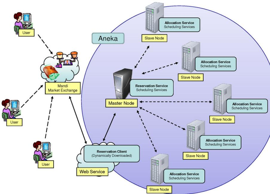
**Fig. 8** The topology of testbed
