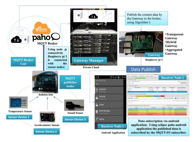
Fig. 6. Tools used for emulating the design Framework.
