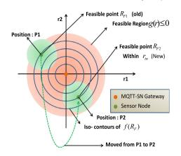
Fig. 3.2b. Inequality constrained state within transaction range, after new sensor node found.
