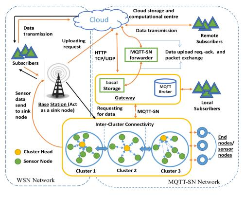
Fig. 1. The existing model of MQTT-SN protocol for WSNs.
