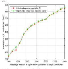
(b) Comparative pub-to-sub delay due to different message payloads for calculative values and real time outcomes by applying the proposed method for QoS level 1  $10^{-2}$
