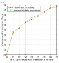
(e) Comparative pub-to-sub delay due to different numbers of packet sending for calculative values and real time outcomes by applying the proposed method in QoS level 1
