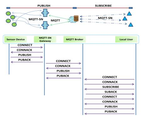
Fig. 4. Estimation of end-to-end delay in QoS-1 level.
