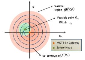
Fig. 3.2a. Inequality constrained state within transaction range, before new sensor node is found.
