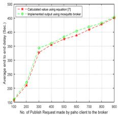
(d) Comparative pub-to-sub delay due to different numbers of packet sending for calculative values and real time outcomes by applying the proposed method in QoS level 0
