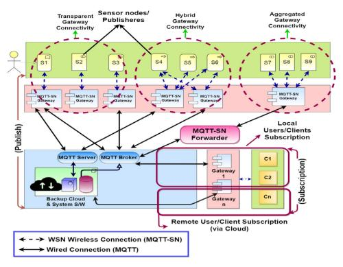
Fig. 2. MQTT-SN gateway architecture.
