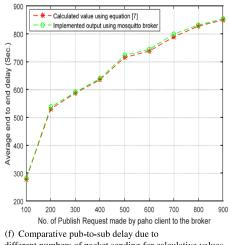
different numbers of packet sending for calculative values and real time outcomes by applying the proposed method in QoS level 2
