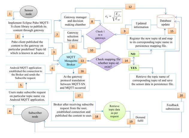
Fig. 7. Workflow of proposed emulation mechanism.
