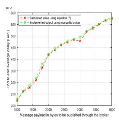
(a) Comparative pub-to-sub delay due to different message payloads for calculative values and real time outcomes by applying the proposed method for QoS level 0
