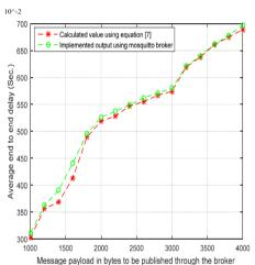
(c) Comparative pub-to-sub delay due to different message payloads for calculative values and real time outcomes by applying the proposed method in QoS level 2
