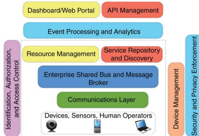
FIGURE 1.3 A Reference Architecture for IoT
