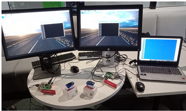
Fig. 6. Real-world implementation of FogBus-based Sleep Apnea analysis.
