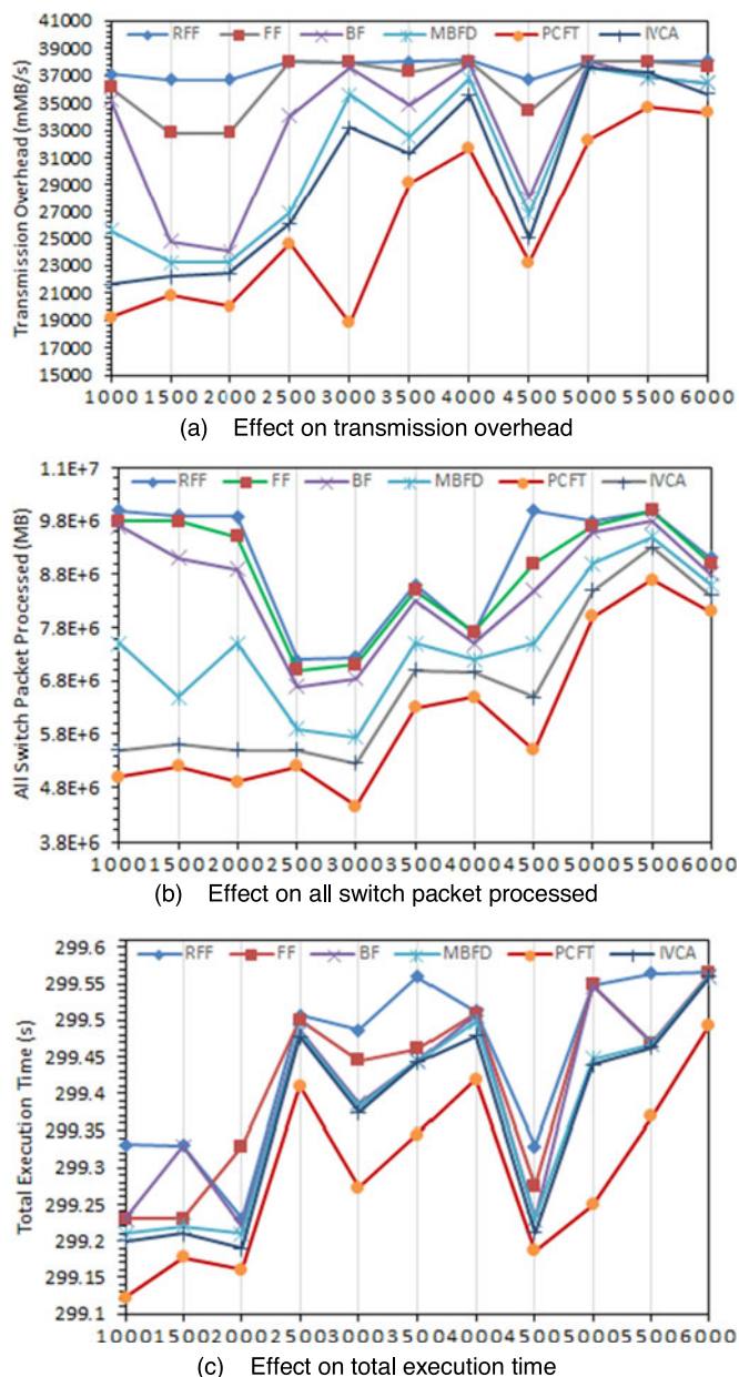
Fig. 11. Effect of number of VMs. The number of VMs represents the number of VMs initially placed. The transmission overhead, all packets routed through all the three layer switches, and total execution time for 1000 parallel applications increase with the number of VMs, but our proposed approach (PCFT) has the lowest growth rate for each figure. (a) Effect on transmission overhead, (b) effect on all switch packet processed, and (c) Effect on total execution time.
