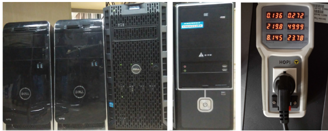
Part of heterogeneous compute nodes Controller node Power meter
