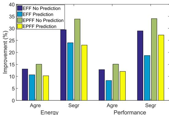
Fig. 3. Percentage improvements in energy and performance using EFF and EPFF placement techniques rather than FF [Boosted Gradient Trees prediction].
