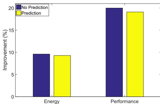
Fig. 2. Percentage improvements in energy and performance using aggregation-based VM placement instead of segregation, using EPPF allocation and EPAM migration [Boosted Gradient Trees prediction].
