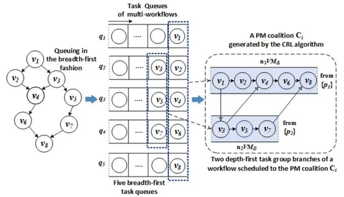
Fig. 3. A case that tasks of a workflow are scheduled to the optimal VM instance bundle  $\mathcal{B}_{c_i}^* = \{n_1 VM_{i1}, n_2 VM_{i2}\}$ .
