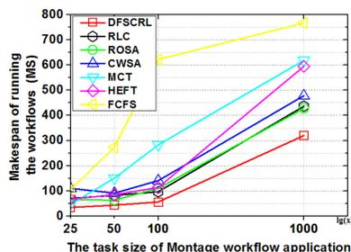
Fig. 8. Makespan of running single type of workflows in the cases of Small (25, 50), Medium (100) and Large (1000) task sizes of Montage workflow applications.
