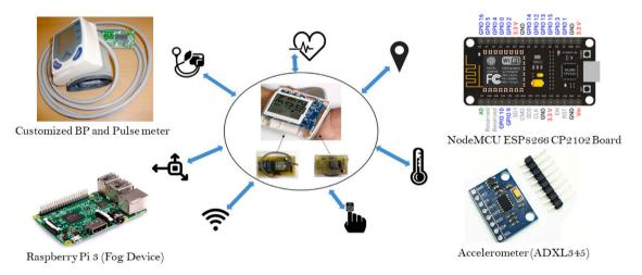
Fig. 6. Low-cost wearable sensor (designed and fabricated in the lab of IIT Kharagpur for this research work).
