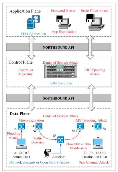
FIGURE 2. Attack vectors at different layers of SDN architecture.
